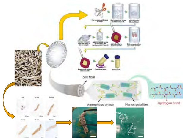
Figure 1. Processes for obtaining native silk structure and regenerative silk fibroin (RSF) [1, 5] (scale bars: 1 cm)
