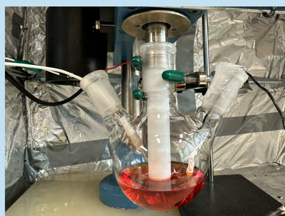
Fig 2. Solution in round bottom flask with electrodes
