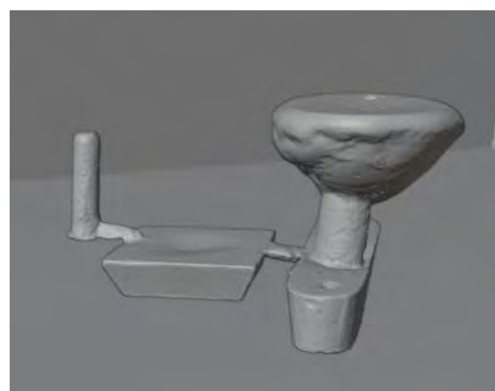
Figure 4 3D scan of sand casted part imported on Blender
