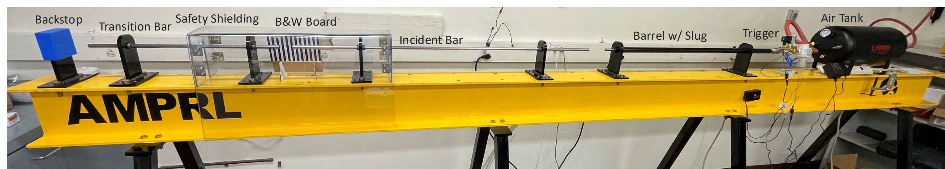
Figure 7 Split-Hopkinson Pressure Bar used for impact testing
