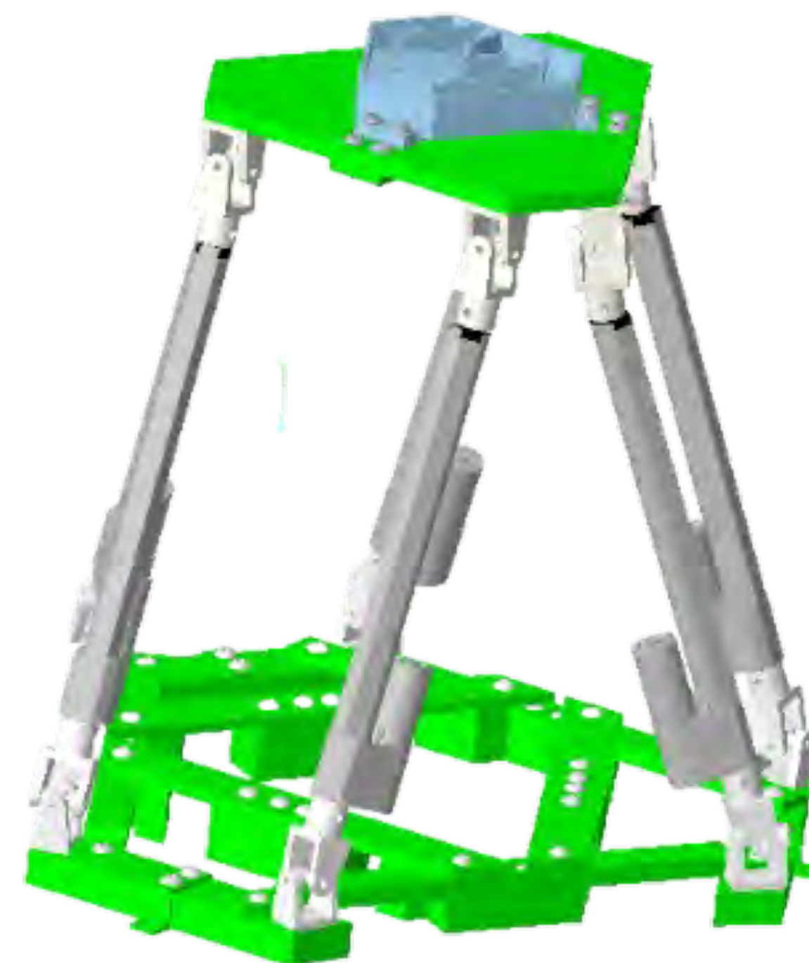
Figure 4 Assembly model of full Stewart Platform set up with attached ball maze.
