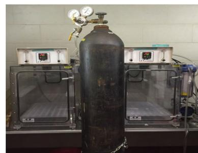
Figure 2: Environmental exposure chambers used to simulate CIH
